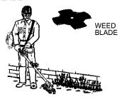
NOTE: Remove the trimmer head and plastic shield before attaching the metal shield and installing the weed blade. To remove the trimmer head, align hole in the dust cup with the hole in the side of the gearbox by rotating the dust cup. Insert a small screwdriver into aligned holes. This will keep the shaft from turning while loosening the trimmer head. Remove the trimmer head by turning
